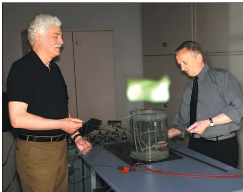
Fire and water Gerd Fussmann and colleagues in Germany have produced this glowing, hovering blob of plasma by simulating the effect of a lightning strike on water. The plasma persisted for about 0.3 s.
